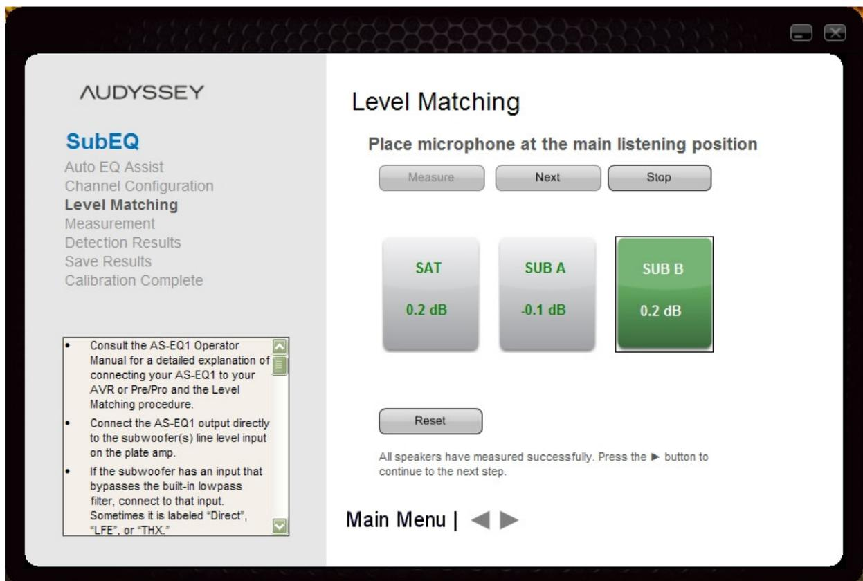
Although similar in appearance to the **Level Matching** Screen in SubEQ 3.1, please note the **Reset** button below the **SAT** and **SUB** measurement boxes. Because SubEQ 3.2 uses a C-weighted Leq measurement method (essentially a running average of the sound pressure level) it is important to note that if you
